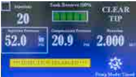
Fig. 9—The warning indicates that the injection port is disabled by default on startup.
