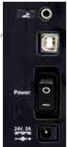
Fig. 3—The foot switch connection, power supply connection and power switch are located on the back panel of the μPUMP.
