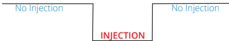
Fig. 14—The injection happens on the high to low transition of the TTL pulse.
