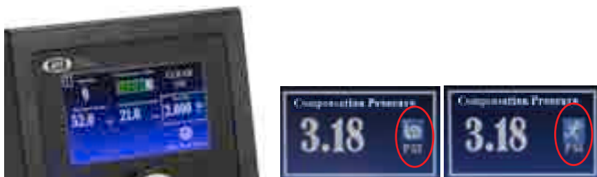
Fig. 17—(Left) Touch the parameter to adjust and rotate the knob to modify the parameter.
