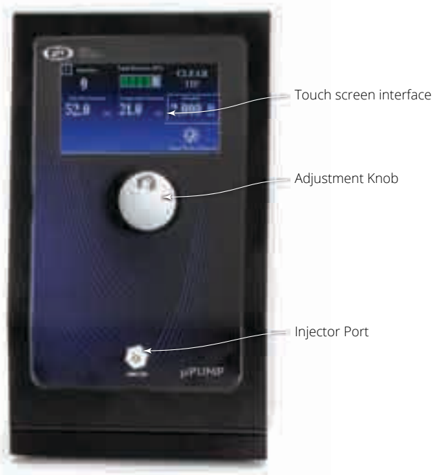
Fig. 2—The major features of the \mu PUMP are labeled in this diagram.
