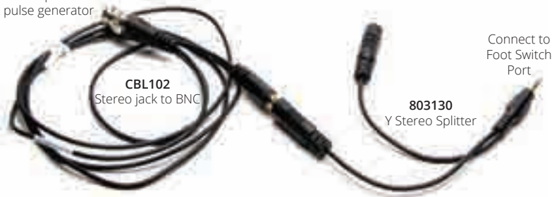
Fig. 13—Use the CBL102 and the 803130 to configure the system for a TTL trigger. The \mu Pump will inject on the high to low transition of the incoming TTL pulse.
