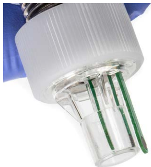
Fig. 8—The outer electrode reaches close to the bottom of the well plate, and the inner electrode does not touch the membrane.
