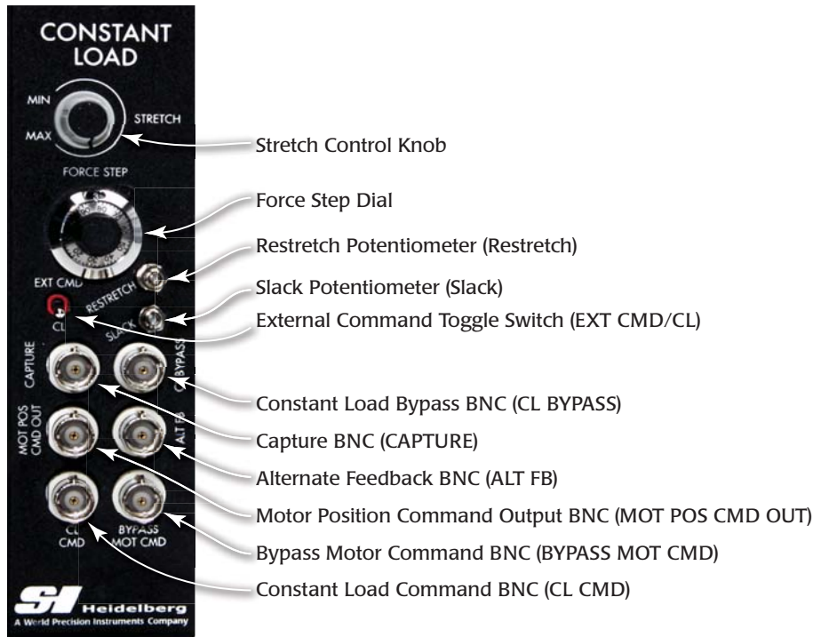
Fig. 20 The SI-COLU Constant Load Module can be used to switch from an isometric to an isotonic contraction by engaging a feedback around a reduced constant measured force.
