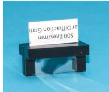
Fig. 34 (Left) The sarcomere grating fits into the cuvette and provides a foolproof calibration method.
