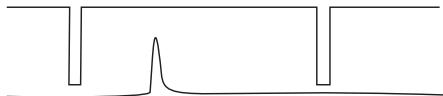
Fig. 36 The top trace shows the timing reference to the video. The camera signal is shown in the bottom trace.
