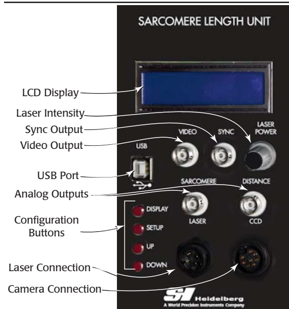
Fig. 14 SI-SARCAM Sarcomere Spacing Module
