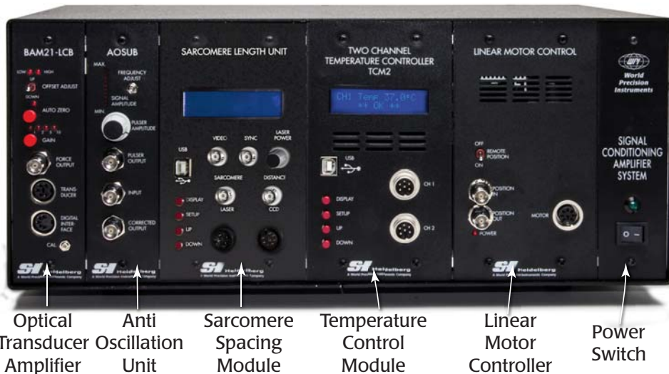
Fig. 4 The front panel of a Signal Conditioning Amplifier System configured for a Muscle Tester shows the SI-BAM21-LCB, the SI-AOSUB, The SI-SARCAM, the SI-MOTDB and the SI-TCMB2.
