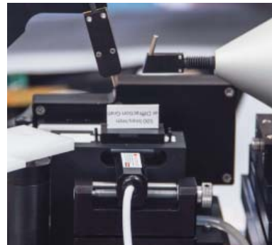
Fig. 34 (Left) The sarcomere grating fits into the cuvette and provides a foolproof calibration method.
