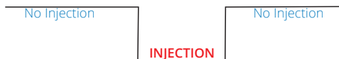
Fig. 15—The injection happens on the high to low transition of the TTL pulse.
