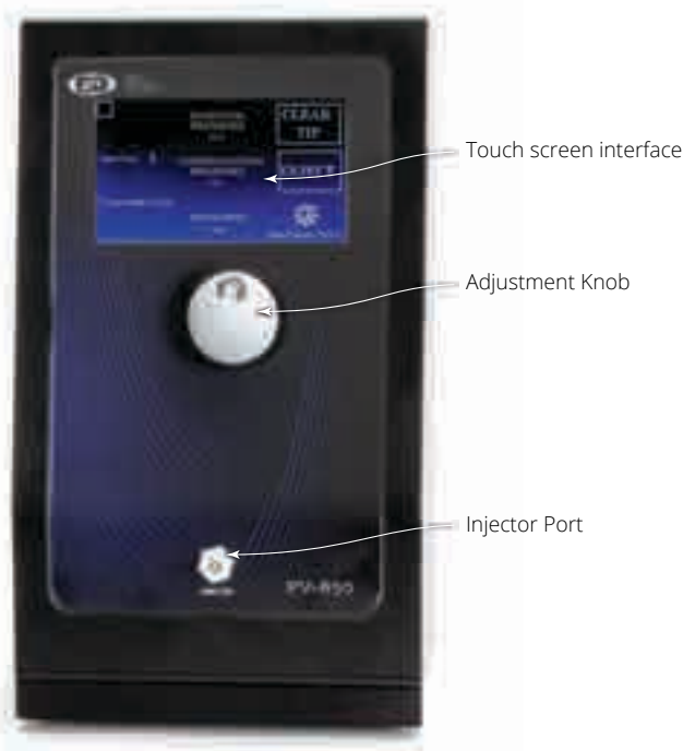
Fig. 2—The major features of the PV850 are labeled in this diagram.
