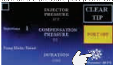
Fig. 16—(Left) Touch the setting area in the bottom right corner to access the Settings menu.
