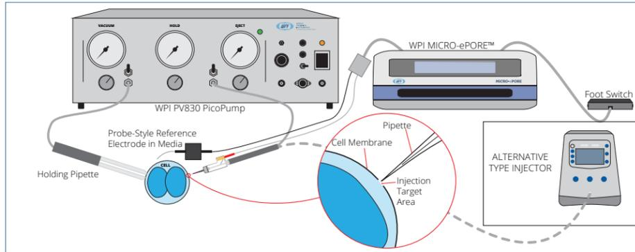
The setup could use the probe-style reference electrode or the well-style electrode, as pictured below.
