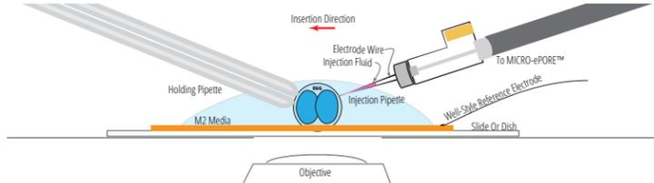
The reference electrode ring is secured to a microscope slide with a vacuum gel, and the media is placed inside the well-style electrode. Both the probe-style electrode and the well-style electrode are included. [Ring reference electrode – OD: 12.7 mm (0.5”), Thickness: 0.4 mm (0.16”)]
