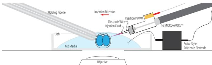
The reference electrode block is positioned near the injection site and the electrode is placed in the electrically conductive media.
