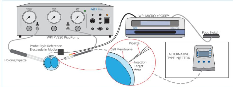
The setup could use the probe-style reference electrode or the well-style electrode, as pictured below.
