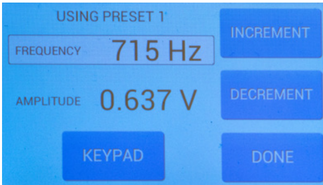
Fig. 18—From the Preset Configuration screen, you may define the frequency and amplitude.
