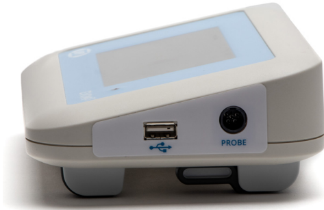
Fig. 3—USB port, Electrode connection
