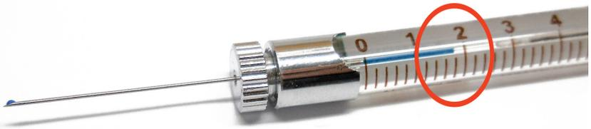
*Fig. 4-Vacuum filling of the syringe leaves an air gap.*
