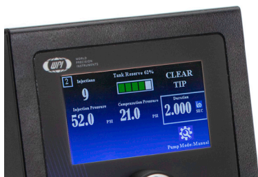
Fig. 17—(Left) Touch the parameter to adjust and rotate the knob to modify the parameter.
