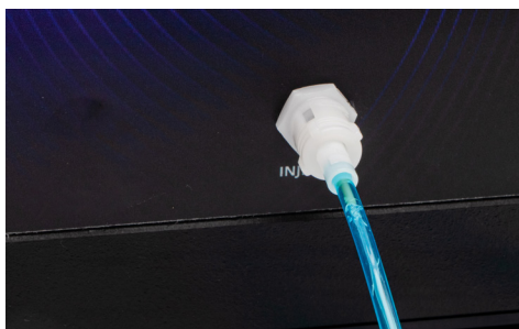
Fig. 11—(Left) Align the connector with the Injection Port, slide the connector in position and rotate the connector a little clockwise to lock it into place.
