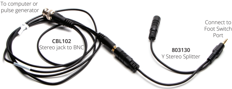
Fig. 13—Use the CBL102 and the 803130 to configure the system for a TTL trigger. The \mu Pump will inject on the high to low transition of the incoming TTL pulse.
