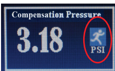
Fig. 17—(Left) Touch the parameter to adjust and rotate the knob to modify the parameter.
