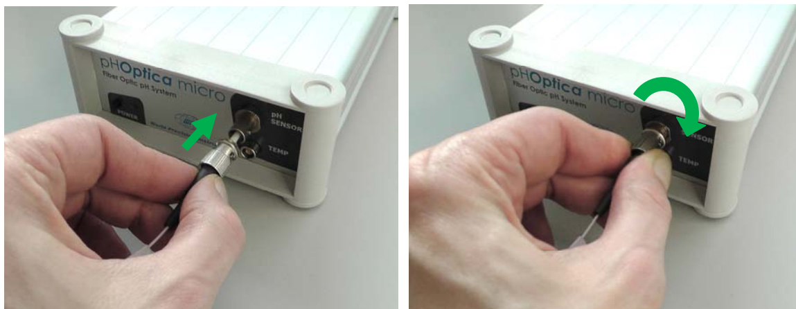
Fig. 6 Attaching the pH microsensor to the connector on the transmitter
