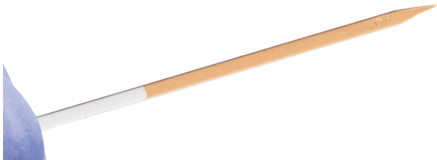
Fig. 1—Inspect the pipette for bubbles, which are seen here at the tip.
