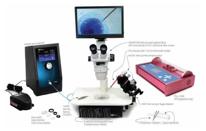
WPI offers a variety of pumps along with special syringes, stereotaxic frames, glass capillaries and needles. The setup you choose depends on the size of your microinjection aliquots, the volume to be injected and the size of needle or glass tip you choose.
