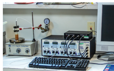
This is a typical laboratory setup of a WPI free radical analyzer with data acquisition system.
