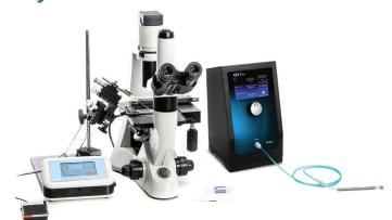
A typical microinjection setup with the MICRO-ePORE™, an INV-101 Inverted Microscope and a PV820 Pneumatic PicoPump.
