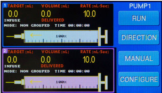
Fig. 15—Channel 1 is selected, and PUMP1 is shown with a blue field behind it in the upper right corner of the display screen.
