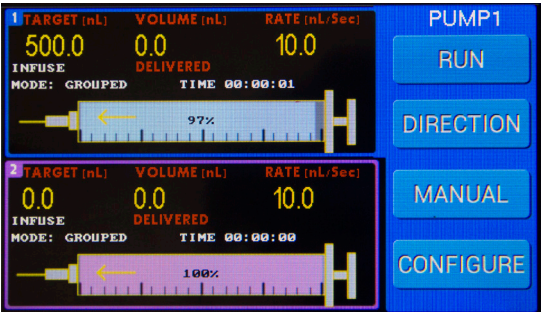
Fig. 12—Channel 1 is selected, and PUMP1 is shown with a blue background. When Channel 2 is selected the background turns pink.
