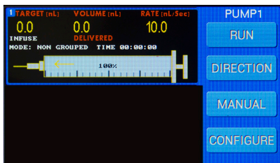
Fig. 30—Only one UMP3 pump is installed, so the second pump display is blank. In this example, Pump 1 is present and Pump 2 is absent. Note that a Nanoliter 2010 will always register as present, whether it is properly plugged in or not.
