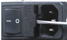
Fig. 6—Insert the screw driver under the fuse housing lip and pry the housing open.
