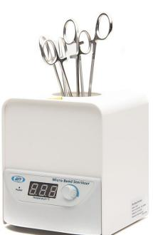
**NOTE**: The top 2.5 cm of beads may not be within the recommended temperature for proper sterilization. To decontaminate 5 cm of an instrument, it must be inserted 7.5 cm into the beads.
