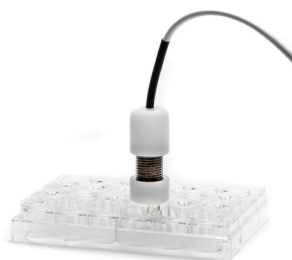
Fig. 12—The STX4 sits securely over a 24-well insert.
