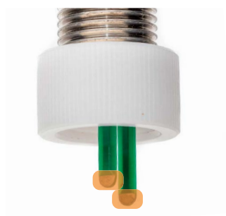
Fig. 33—Verify the electrode sensing tips (highlighted region) on both blades stay fully immersed in a conductive liquid (cell culture media or buffer) during measurement. You need to have adequate apical and basolateral volumes to get a stable reading.
