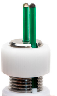
Fig. 32—The darkening of the STX4 electrode tip and a significant difference in color between inner and outer sides of the electrode blades (during storage or after a period of use) are considered normal.
