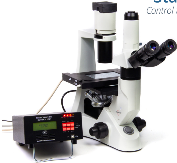
The ECU is positioned on an inverted microscope. The ECU system consist of the stagetop environment base unit and the electronic controller.
