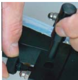
Fig. 30–(Left) Clamp for cable of the temperature sensor.
