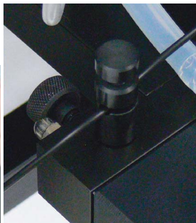
Fig. 30–(Left) Clamp for cable of the temperature sensor.
