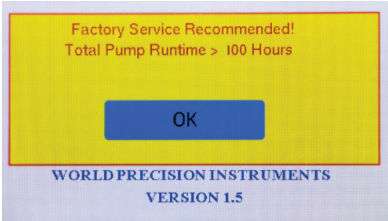
Fig. 29—Warning errors like this one display when the unit needs to be returned to the factory for routine service.
