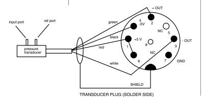
pin connector are shown below. This connector is compatible with **Transbridge** (WPI Part #TBM4M), a four-channel amplifier transducer manifold, and **Bridge-8** (rack-mountable amplifier modules). If the user wishes to rewire the transducer to a different plug, the colorcoded wires should be connected to conform to the required DC voltage, polarity and signal output connections as shown.
