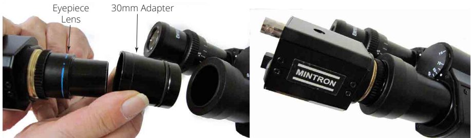
Fig. 72—Camera mounted in eyepiece
