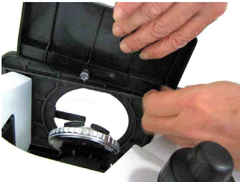
Fig. 14—Left stage plate captive screws
