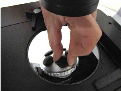
Fig. 38—Removing dust cover to mount objective
