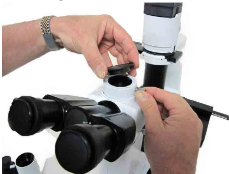
Fig. 32—Remove dust cover
