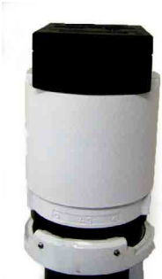
Fig. 24—Assembled condenser with lamp housing
