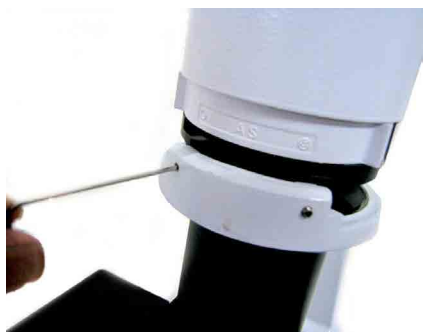
Fig. 20—Tighten hex screws on condenser head
