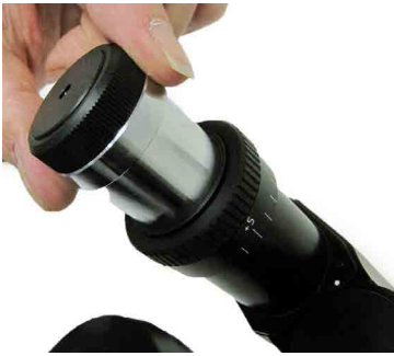
Fig. 61—Phase telescope in eyepiece
