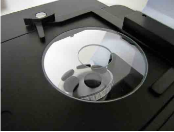
Fig. 25—Clear stage plate, installed
