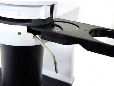
Fig. 65—Insert hex wrench in the right opening
