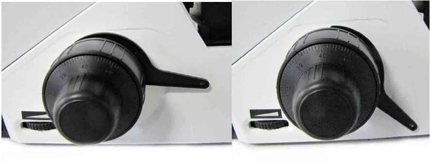
Fig. 81—Tension Adjustment Tool installed
