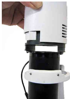
Fig. 18—Condenser in mounting position
