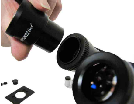
Fig. 51—Placement of eyepieces
