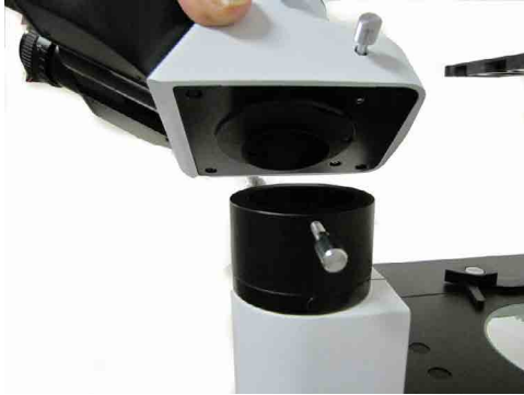
Fig. 30—Position head on the mount
