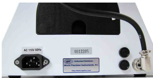
Fig. 4—Back of the microscope base showing power connection, serial number and fuse compartment
