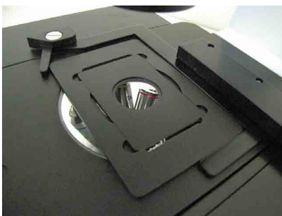
Fig. 48—Placement location of the assembled stage plate
