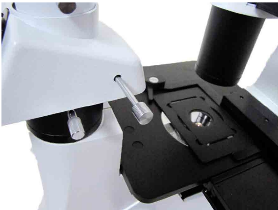
Fig. 77—Switch to enable trinocular extension viewing
