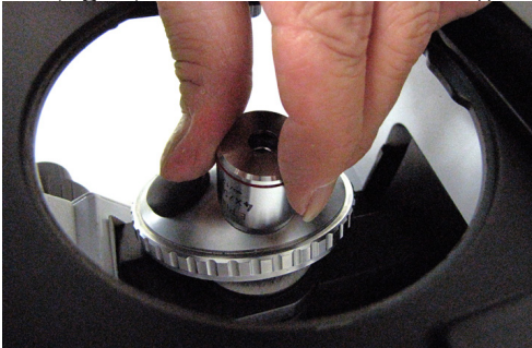
Fig. 42—Installing the objective
