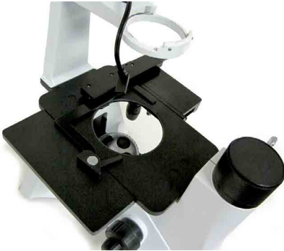
Fig. 16—Coaxial and left stage plate mounted
