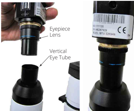
Fig. 70—Line up the camera with tube
