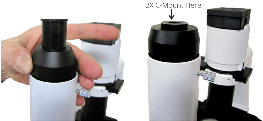
Fig. 34—Eyepiece tube screw mounted
