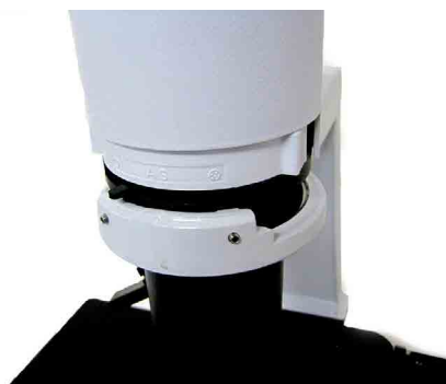
Fig. 18—Condenser in mounting position
