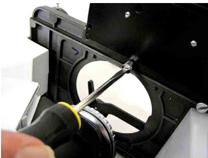
Fig. 10— Fig. 10 —Gently tighten the captive mounting screws.
