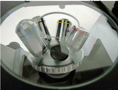
Fig. 45—Clear stage plate in place
