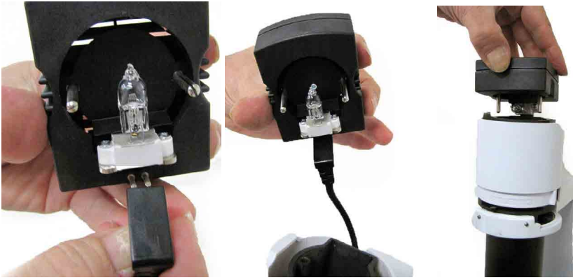
Fig. 21—Connect the lamp
