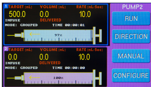
Fig. 54—Pump 2 is the Master pump, and Pump 1 is the slave in this example.
