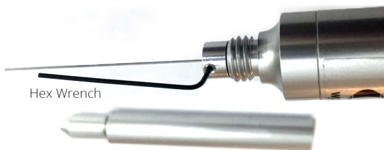
Fig. 47—Loosen the set screws with the hex wrench.
