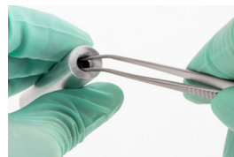
Fig. 14— (Right) Use the tweezers to remove the gasket from the aluminum barrel.
