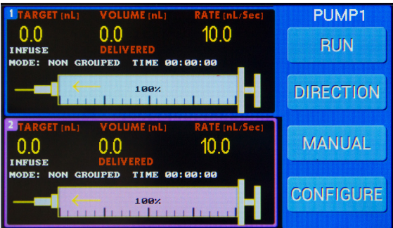
Fig. 18—Channel 1 is selected, and PUMP1 is shown with a blue field behind it in the upper right corner of the display screen.
