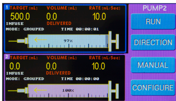
Fig. 41—Pump 2 is the Master pump, and Pump 1 is the slave in this example.
