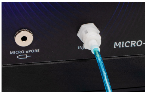
Fig. 12—(Left) Align the connector with the Injection Port, slide the connector in position and rotate the connector a little clockwise to lock it into place.
