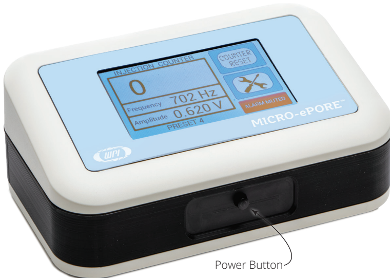
Fig. 2—The power button is on the front face of the MICRO-ePORE™ unit.
