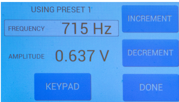
Fig. 16—From the Preset Configuration screen, you may define the frequency and amplitude.
