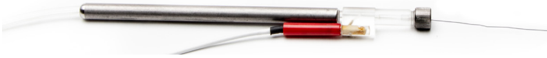
Fig. 8—The red pin of the microelectrode interface cable connects to the microelectrode holder.
