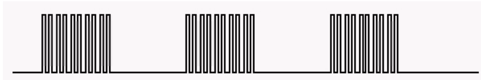
Burst of pulses separated by InterTrain Durations.
