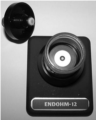
Fig. 6—(Left) A clean EndOhm surface with no spots or irregularities Fig. 7—(Right) Notice the center tip and the small ring on the top section. These may require the use of a cotton swab to clean.
