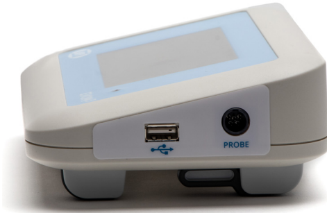
Fig. 3—USB port, Electrode connection
