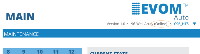
Fig. 15—The online/offline state of the system displays next to the electrode array type in the header on the right side of the window.
