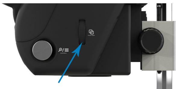
Fig. 20—Use the 3D Adjustment dial to fine tune the depth of field.
