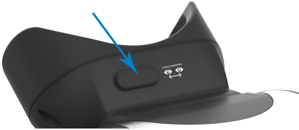
Fig. 11—Adjust the interpupillary distance slider to move the eyepieces closer or further apart to match the spacing of your eyes.
