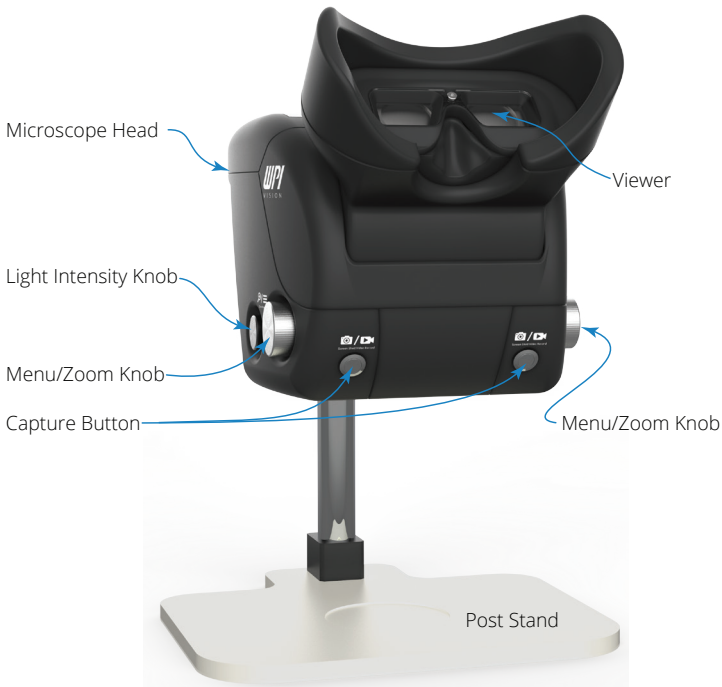
Fig. 2—The knobs and dials on the front face of the scope are labeled. Here the scope is mounted on a Post Stand.
