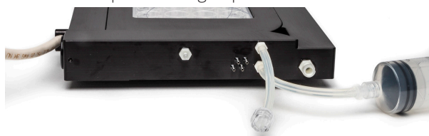
Fig. 15—Connect the syringe to the blue connector on the filling tube.
