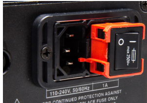
Fig. 60—(Left) Insert the screw driver under the fuse housing lip and pry the housing open. Fig. 61—(Right) The fuse housing slides out.
