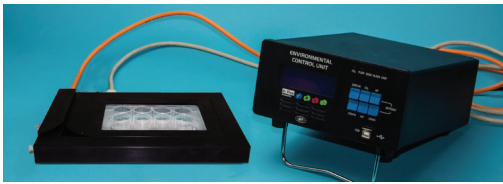
Fig. 1—The Stagetop Environment (STEV) and ECU (Environmental Control Unit) comprise the basic incubator system for growing cells under controlled conditions.
