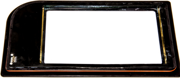
Fig. 21—The rounded corner of the lid fits into the thumb hold on the base of STEV. Notice the electronic interface connection in the bottom left corner of the image. This interface allows the controller to communicate with the lid and control the lid temperature.
