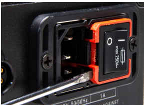
Fig. 60—(Left) Insert the screw driver under the fuse housing lip and pry the housing open. Fig. 61—(Right) The fuse housing slides out.
