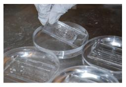
Allow the agarose to solidify, then remove the mold.
