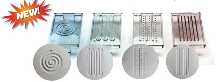
Improve your process time and accuracy by molding your agar plates. Are you looking for a simplier method for handling zebrafish embryos? To speed up your process and accuracy, try **Z-MOLDS**. Mold your agarose, pipette in your embryos, and watch them auto aligning in the grooves.
