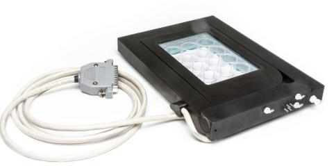
(Above) All the connection ports for the STEV are located on the same side of the unit.
