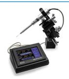
Microprocessor-controlled Nanoliter Injector NANOLITER2020 with SMARTouch controller uses positive displacement injection, eliminating the need for pipette calibration. System uses glass micropipettes.
