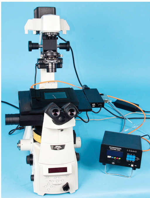
The Environmental Control Unit is positioned on an inverted microscope for a simple live cell imaging setup.
