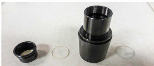
Fig. 29—The reticle ring was removed.
