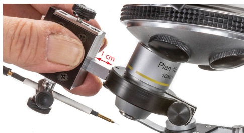
Fig. 7—Mounting the Filament Adjustment Assembly
