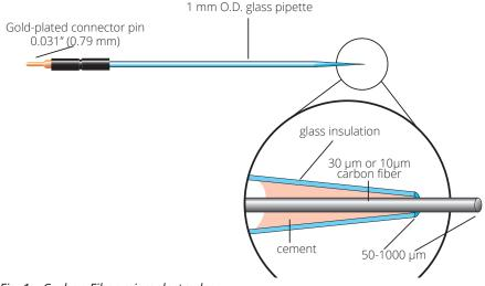
Fig. 1—Carbon Fiber microelectrodes
