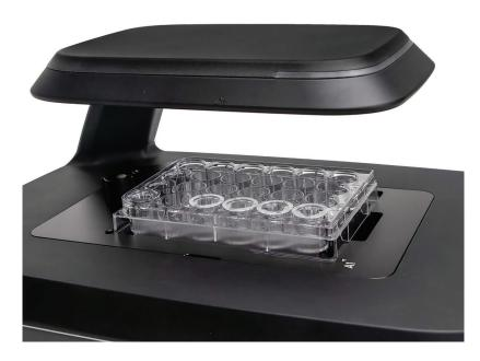
monitored in real time after treating the cell with or without nocodazole using EVOM™ AutoLCI, a live cell imaging device.
