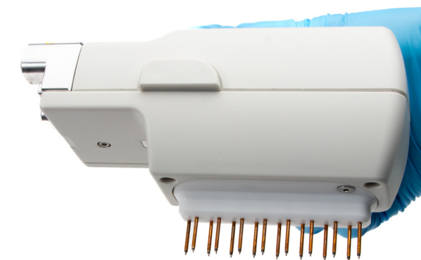
The EVA-EL-03-01 electrode array has 8 pair of (1.25mm Φ) electrodes, which are specially designed to fit precisely in 96 transwell plates, ensuring consistent placement. It performs resistance measurements directly in the plate, common or divided, reducing the possibility of contamination and mechanical damage to your cultured cells.
