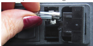
Fig. 3—Open the fuse housing and rotate it right to remove the fuse.
