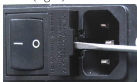
Fig. 2—Insert the screw driver under the fuse housing lip and pry the housing open.
