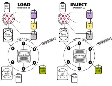
In inject mode the sample loop is included in the fluid flow path, and the pump pushes solution through the sample loop and the sample cell.
