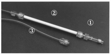
The PicoNozzle holds a microinjection pipette during microinjection. It features good stability, minimum dead volume for fast response, and allows pipettes to be changed quickly and easily.
