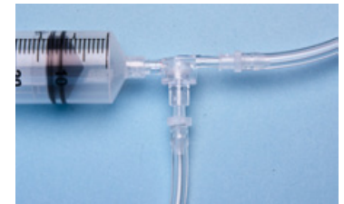
Fig. 3—The inlet tubing enters from the bottom, and the outlet tubing exits to the right side.
