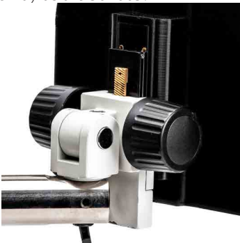
Fig. 21—The 505610 focus mount at the end of the 505606 boom stand has the Enhanced Reality Macroscope mounted on it.
