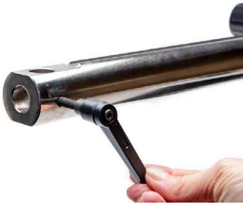
Fig. 13—Screw the clutch handle into position at the end of the horizontal bar.
