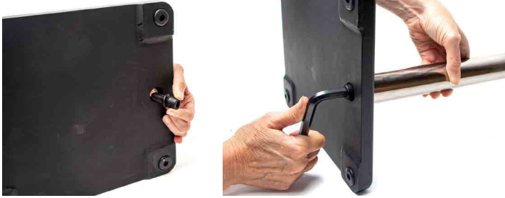
Fig. 3—(Left) Put the locking washer on the anchoring screw and insert it through the hole on the bottom of the base into the threaded hole in the bottom of the vertical post.
