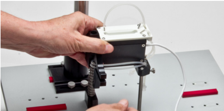
Fig. 4—The Cuvette is installed.
