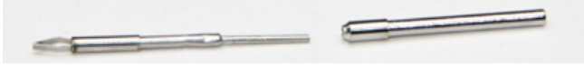
Fig. 9—The mounting hook slides into the adapter before it is installed in the micrometer assembly.
