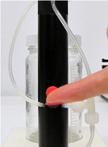
Fig. 26—Lift the spring-loaded pinch valve to allow the waste fluid to be evacuated into the reservoir
