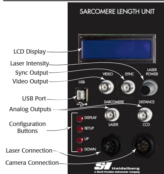
Fig. 13 SI-SARCAM Sarcomere Spacing Module
