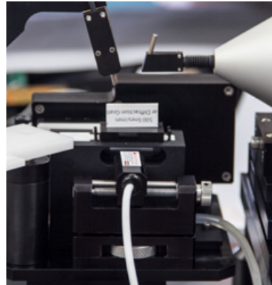
Fig. 32 (Left) The sarcomere grating fits into the cuvette and provides a foolproof calibration method.
