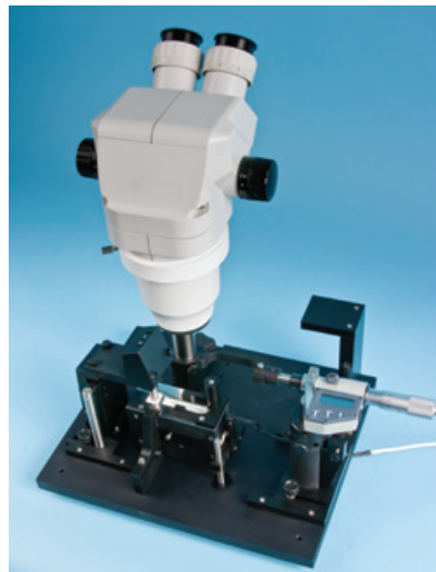
Fig. 1 (Left) SI-MT is a convenient platform for all standard mechanical experiments on intact muscle preparations.
