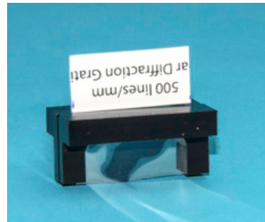
Fig. 32 (Left) The sarcomere grating fits into the cuvette and provides a foolproof calibration method.
