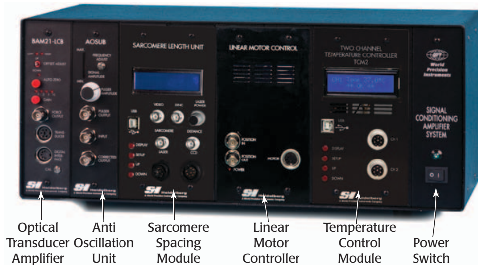
Fig. 4 The front panel of a Signal Conditioning Amplifier System configured for a Muscle Tester shows the SI-BAM21-LCB, the SI-AOSUB, The SI-SARCAM, the SI-MOTTEST and the SI-TCMB2.
