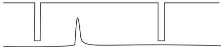
Fig. 34 The top trace shows the timing reference to the video. The camera signal is shown in the bottom trace.
