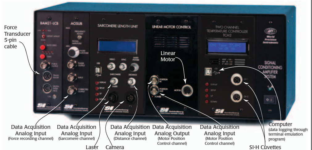
Fig. 18 Connect the system as shown above.
