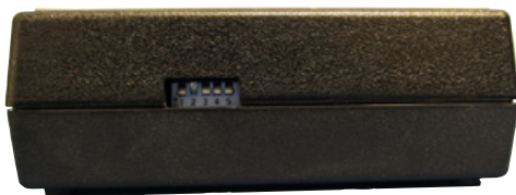
Fig. 3 —The right side of the controller box has five DIP switches for controlling aliquot injection volumes and injection speeds
